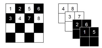
Figure 3: Masking schemes for affine coupling layers. On the left, a spatial checkerboard pattern mask. On the right, a channel-wise masking. The squeezing operation reduces the  $4 \times 4 \times 1$  tensor (on the left) into a  $2 \times 2 \times 4$  tensor (on the right). Before the squeezing operation, a checkerboard pattern is used for coupling layers while a channel-wise masking pattern is used afterward.
